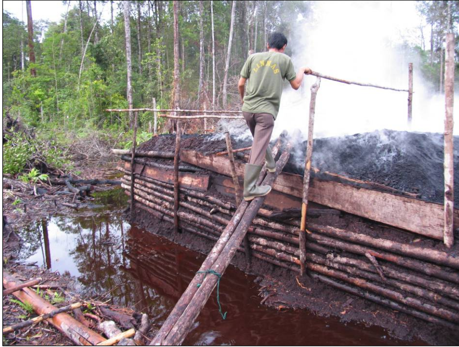
Photograph of a charcoal kiln in operation at the edge of secondary forest, Haparing Hurung.
