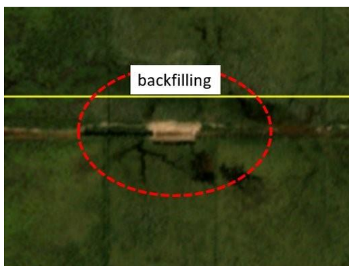
Figure 2.5. Example of the use of high-resolution satellite data for monitoring canal blocking and canal backfilling
