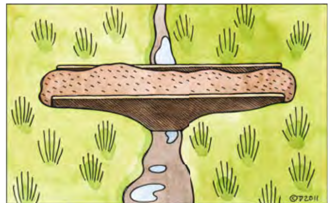
Figure 39. Dams made of plywood can be used to block shallower ditches. Board should be sawn to sizes with greater length and depth than the ditch. To put them in place grooves can be cut in the peat using a long-reach motor-saw. The boards can then be hammered into place e.g. with a sledgehammer. Peat should then be shovelled in between the boards and packed tightly. ILLUSTRATIONS: TUPU VUORINEN.
