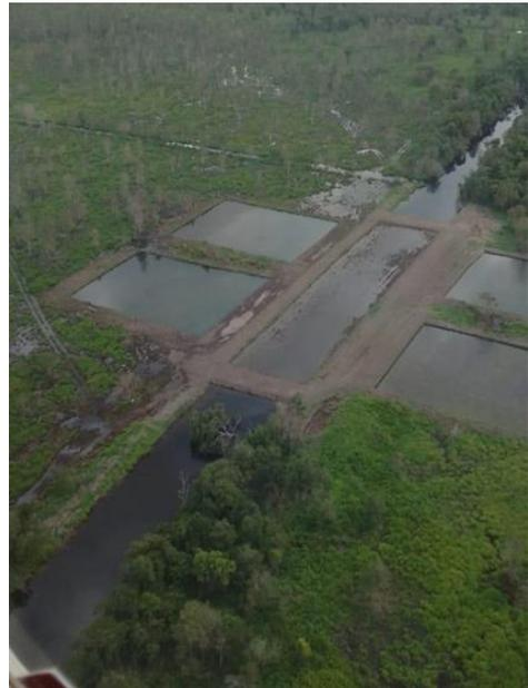
Gambar 7.2 Penimbunan Kanal (Canal Back Filling)
