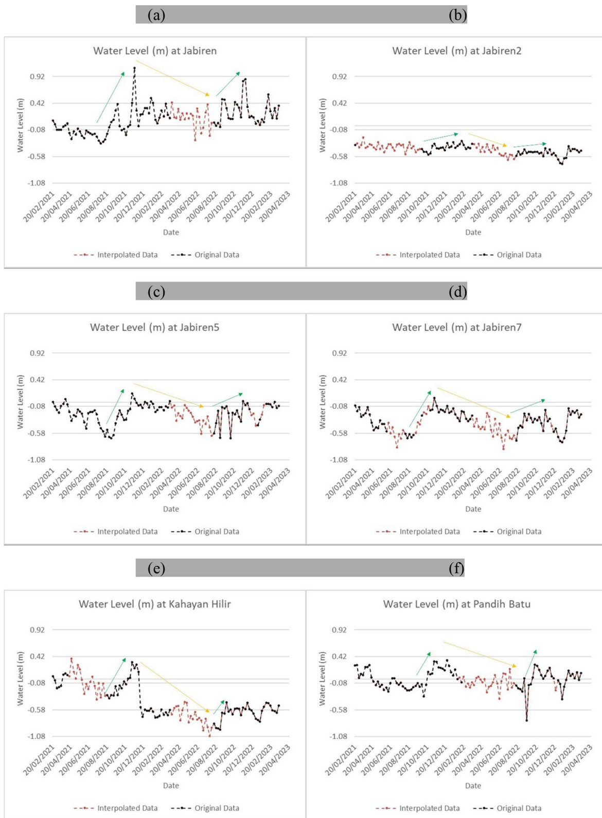
Fig. 4 Water level graphs in meters of the original data (black) and the interpolated results (red) for Jabiren (a), Jabiren2 (b), Jabiren5 (c), Jabiren7 (d), Kahayan Hilir (e), and Pandih Batu (f). The green arrows show an increasing trend, while the orange arrows show a decreasing trend
