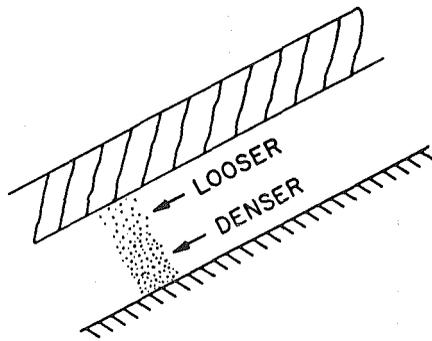
**FIG. 6.—Example of Potential Situation for Mechanism B Failure Arising from Rearrangement of Soil Into Looser and Denser Zones**
