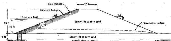
FIG. 2.—Cross Section through Sheffield Dam at Time of Failure
