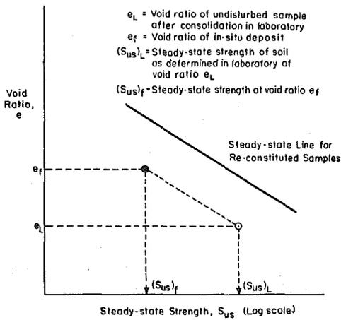
**FIG. 4.—Procedure for Determining Steady-State Strength for Soil at Field Void Ratio Condition (after Poulos, et al. 1985)**
