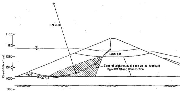
FIG. 1.—Cross Section of Lower San Fernando Dam at End of Earthquake
