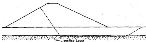
FIG. 7.—Schematic View of Low Embankment Underlain by Very Loose Sand Layer
