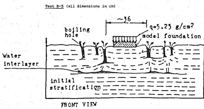
**FIG. 5.—Results of Shaking Table Test on Deposit of Stratified Sand (after Liu and Qiao, 1984)**
