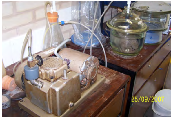
Figure 6-17 Vacuum pump and desiccator used to saturate concrete specimens
