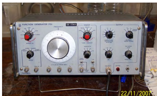
Figure 6-20 A.C. Signal generator used to measure resistivity
