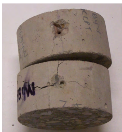
Figure 11-18 BPD sample cracked during drilling
