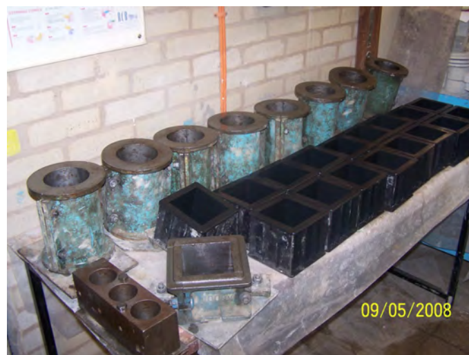
Figure 11-3 Pre-oiled moulds before casting
