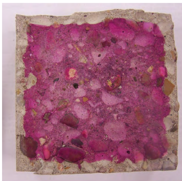
Figure 11-22 Carbonation depth in sample BPD-GGBS-BOS (w/b=0.5, water cured)
