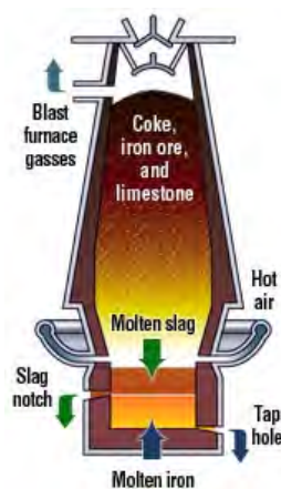
Figure 2-1 Iron blast furnace
