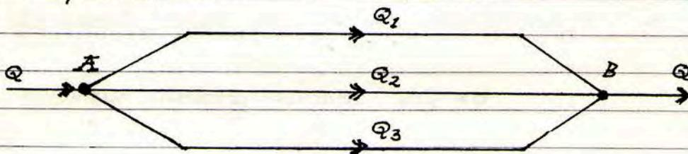
$$Q = Q_1 + Q_2 + Q_3 \quad \text{dan} \quad h_{L(AB)} = h_{L_1} = h_{L_2} = h_{L_3}$$
