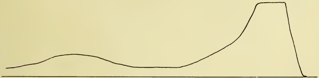
LEAK 149 FEET FROM THE VALVE.
