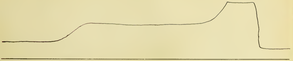
LEAK 149 FEET FROM THE VALVE.
