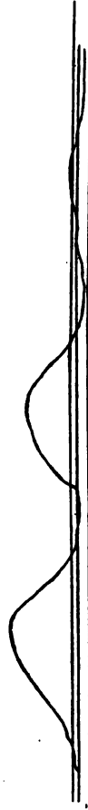
FIG. 22. Diagram taken between the Air Chamber and the Origin. INDICATOR DIAGRAMS IN THE CASE OF A SMALL AIR CHAMBER.
