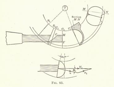
through the angle  $B_1OC_3$ . The average value of  $\alpha_1$  will be taken as the angle obtained when the bucket occupies the mean between these two extreme positions. It is evident that position  $C_3$  will depend upon the speed of the wheel, and that the faster the wheel goes the farther over will  $C_3$  be. Thus the angle  $\alpha_1$  decreases as the speed of the wheel increases. The variation in the value of  $\alpha_1$  as worked out for one particular case is shown in Fig. 85.
