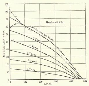
Fig. 86.—Relation between torque and speed.
