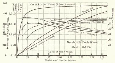
Fig. 89.-Nozzle coefficients and other data.
