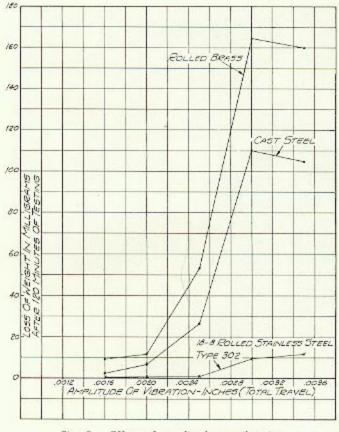
Fig. 5 — Effect of amplitude on vibration.
