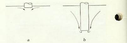
Fig. 17—Flow of liquid below test specimen according to Rightmire.
