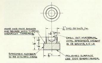
Fig. 3—Buttons used for test specimens in cavitation machine.
