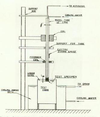
Fig. 1—Schematic layout of vibratory type accelerated cavitation machine.
