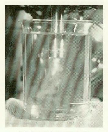
Fig. 9—Photograph of specimen vibrating in oil.
