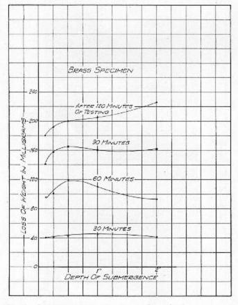
Fig. 6—Cavitation tests to determine effect of submergence on brass specimen. reasons why the depth of pitting decreases with a decrease in amplitude is apparent when observing the test fluid in stroboscopic light. As the amplitude is decreased the size of the vapor bubbles that form beneath the button also decrease. According to the theory of collapse of a vapor bubble, the smaller the bubble the smaller the velocity of collapse and therefore the smaller the pressures produced.
