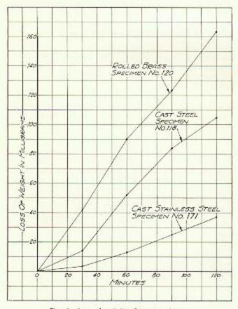
Fig. 4-Loss of weight of test specimens.
