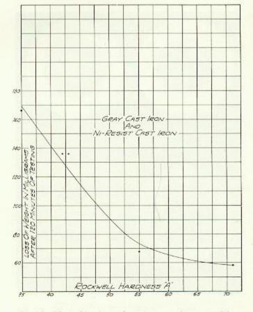
Fig. 10—Effect of hardness of cast iron on resistance to pitting.
