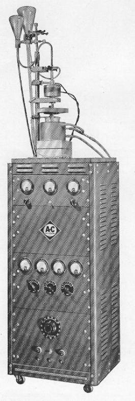
Fig. 2-Photograph of accelerated cavitation test machine.
