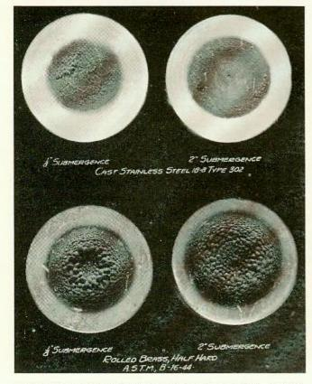
Fig. 8—Photograph of brass and stainless steel at  $\frac{1}{8}$  in. and 2 in. submergence.
