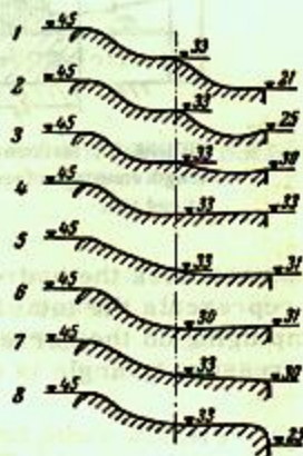
FIGURE 62. Influence of configuration and level of end sill on ejection effect.
