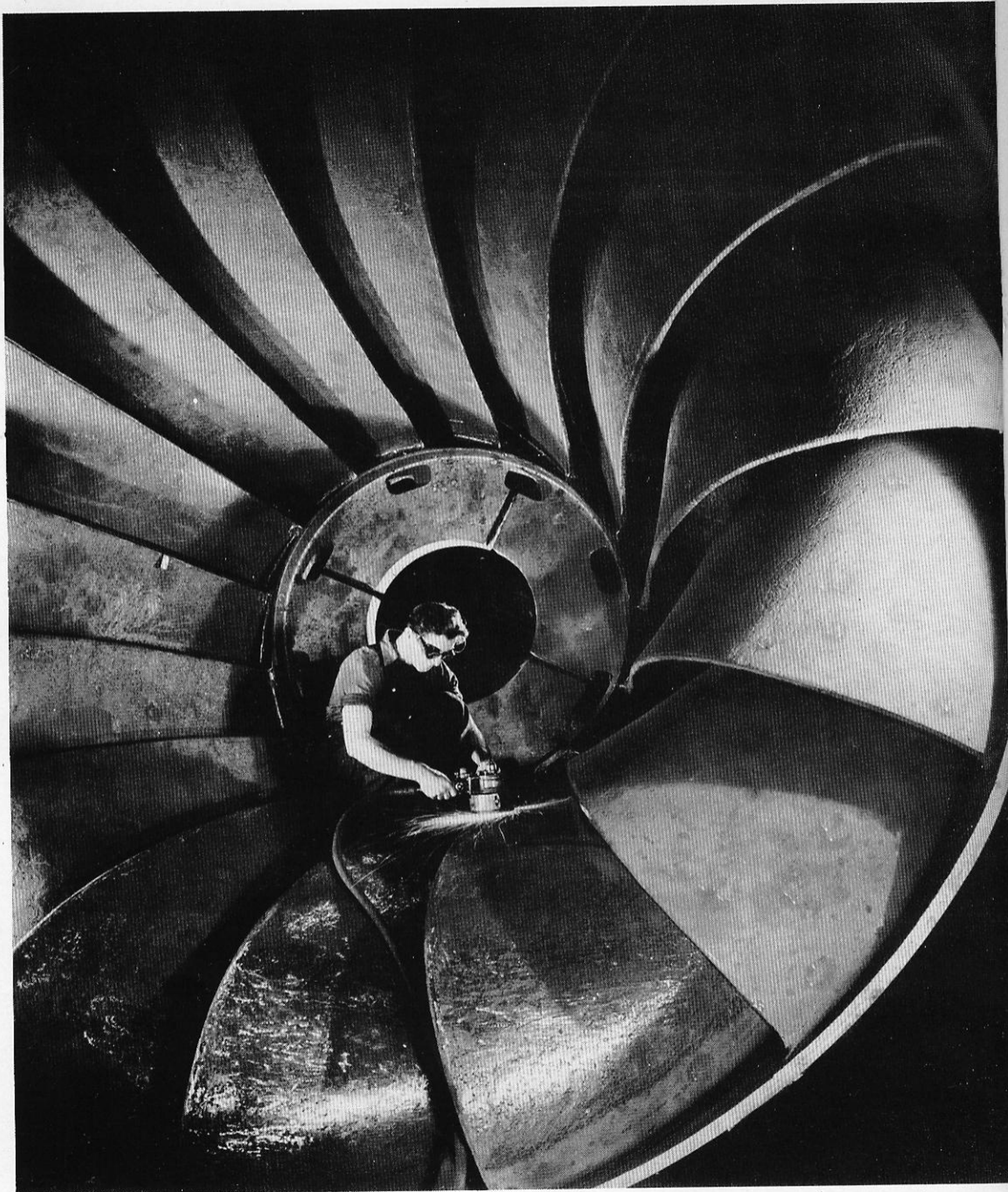
Finish machining gives a glass-smooth surface to the runner for a 35,000 hp Francis type hydraulic turbine destined for TVA.
