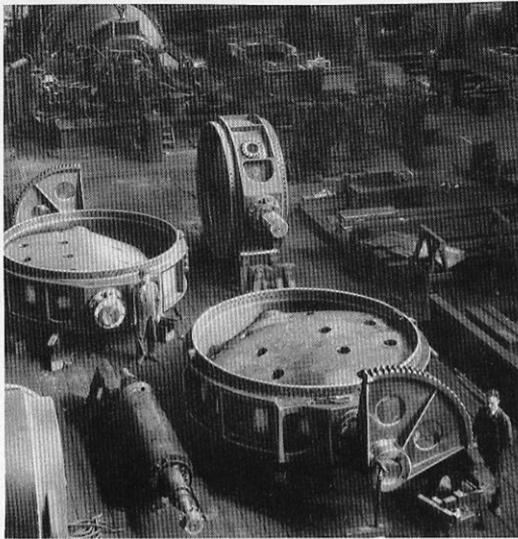
Fig. 17 — One 11 and two 9 foot butterfly valves for two 39,000 hp vertical steel plate spiral cased turbines.
