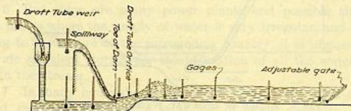
FIG. 2 DESIGN OF TESTING FLUME
